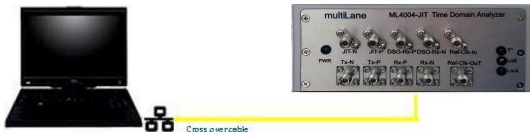
Figure 40: ML4004-JIT Rev B connected with Ethernet crossover cable
